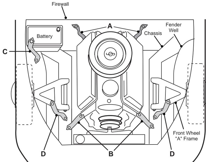
Figure 10-5. Ground Bonding
