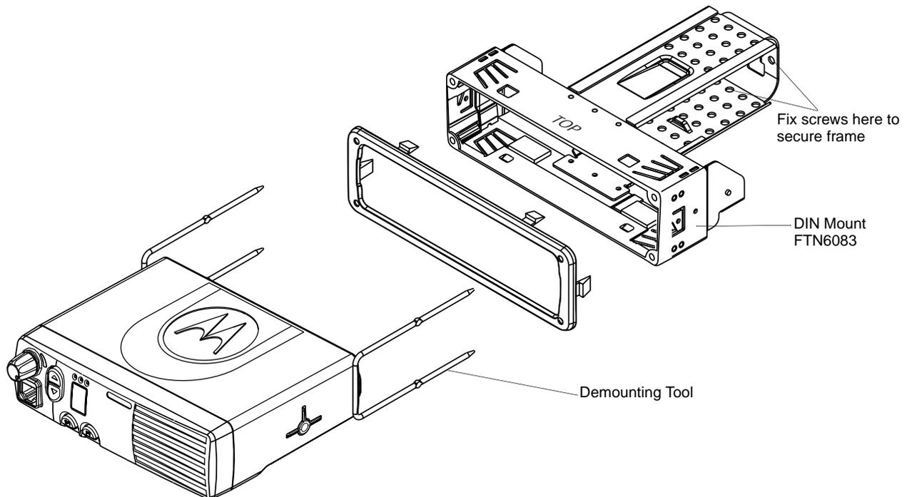
Figure 5-1. Fitting the Radio into the Frame
